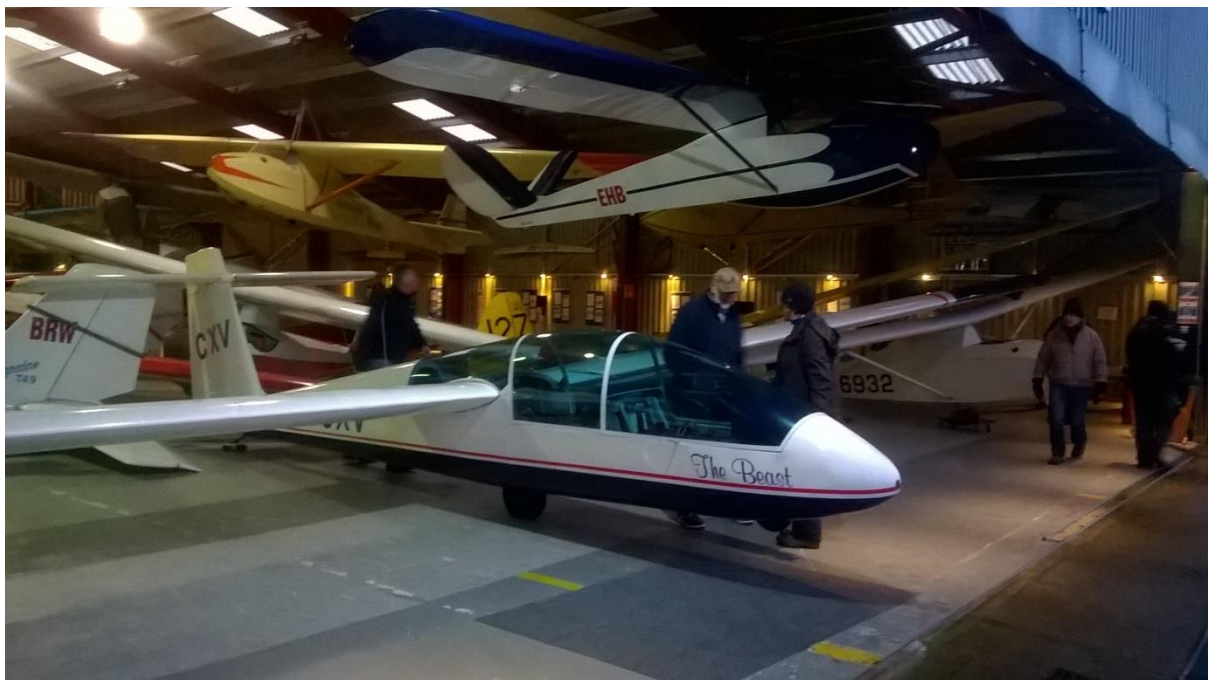
The YS53 "Beast" in its new home alongside a Capstan and a Grunau, above it is a K3 (V tail) fore-runner to the K8 and the first glider with a metal tube fuselage.
